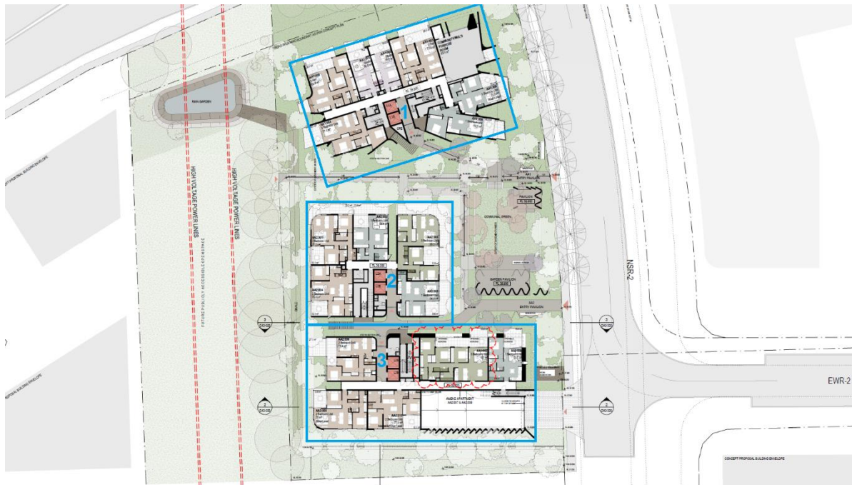
Figure 6. Proposed ground floor plan (overlaid with blue lines defining 3 lift cores and the units they access).
